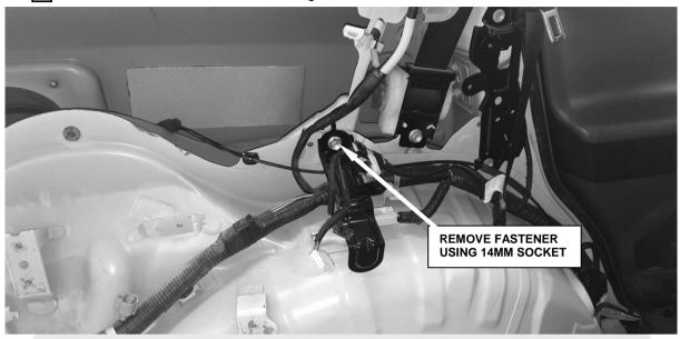
Retain fastener and set bracket aside. Image below shows the 4 attachment points for compressor bracket
