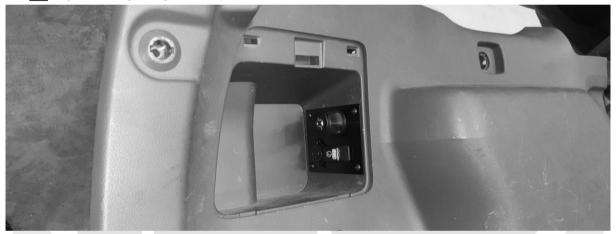
Secure switch plate to trim panel using 4X M6X16 Button Head Screws, 4XM6X16X1.2 washer and M6 Nyloc Nut.
